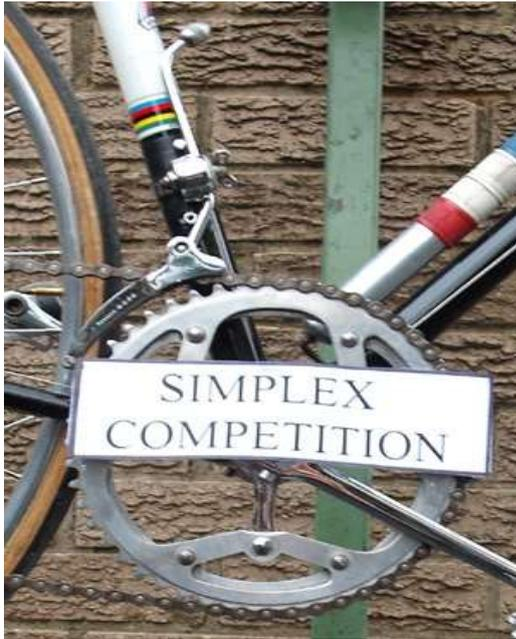
had toe clips and straps, brake cables were all on show and gear levers were on the down tube for the rear mech, with a lever on the seat tube for the front changer (see picture). The block (now a cassette) had 5 sprockets and with a double clanger (double chainset).
